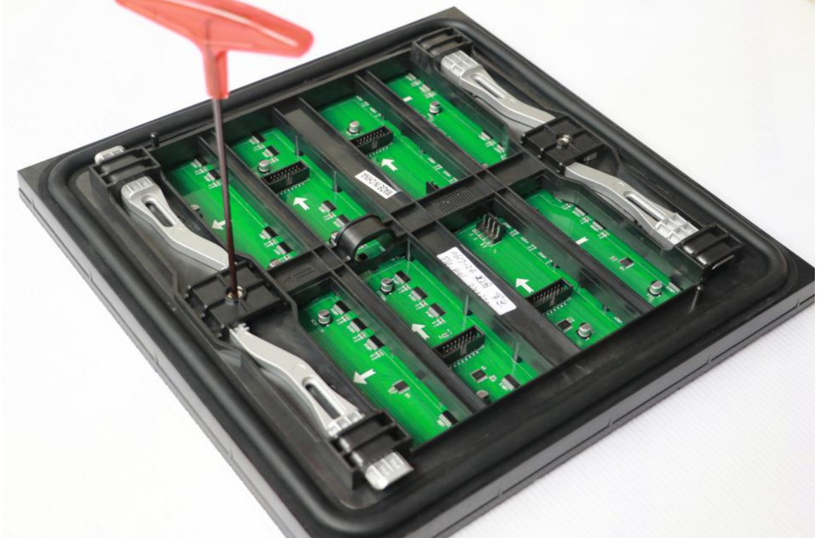
P10 SMD 32X32 LED Module Back View
